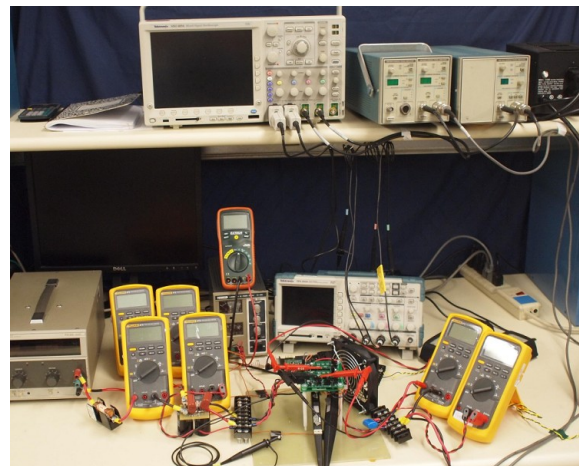
Fig. 8. Setup used to test the GaN HEMT switched-capacitor.
