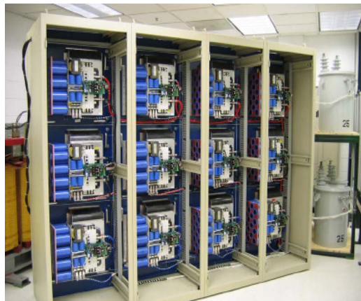
Fig. 9. Cascade multilevel inverters of 1 MVA.
