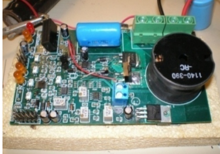
Fig. 11. 250 Watt dc/dc converter used to drive the TEC module.
